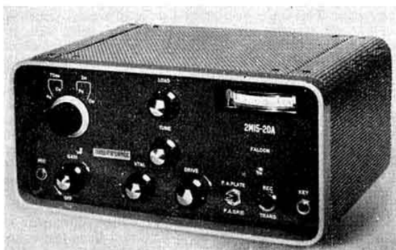
The Green and Davis 2M15-20A "Falcon" is a 20 watt input phone and c.w. transmitter for 2m for operation from 230V a.c. or 12V d.c. A switched 250V d.c. supply for an associated receiver is provided. The "Falcon" has also push-to-talk facilities and internal switching and controls for operating an external 70cm tripler/amplifier. Cabinets in the same style can be supplied at £12 each.
